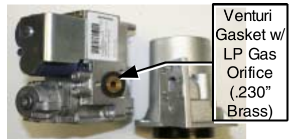
Gas Control with .230" LP Orifice
